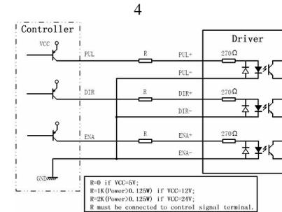
Figure 3: Connection to PNP signal (common-cathode)
