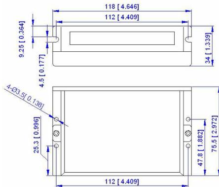
Figure 1: Mechanical specifications
