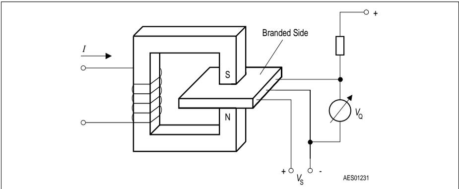
**Figure 5 Sensor/Magnetic-Field Configuration**
