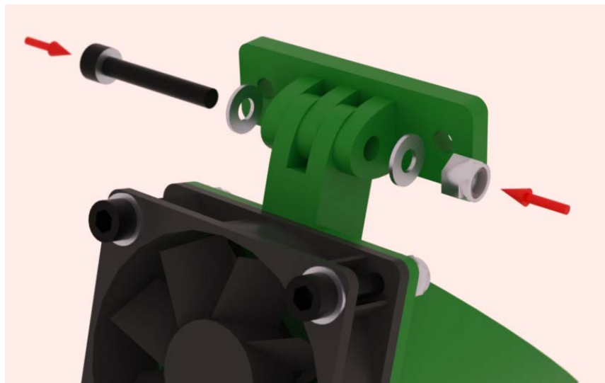
Figure 37: Part Cooling Fan and Swivel Bracket Assembly
