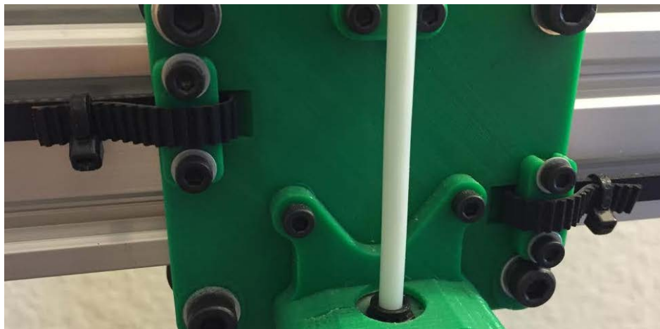
Figure 53: Core-XY Belt clamps
