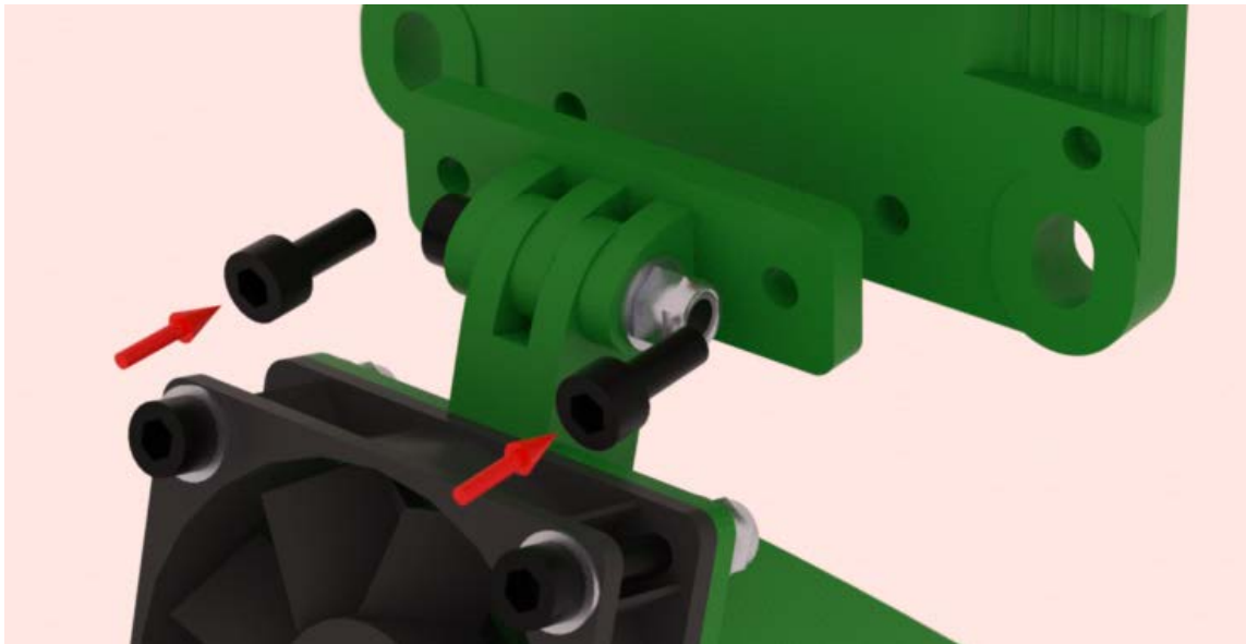
Figure 38: Part Cooling Fan Swivel Mount Assembly
