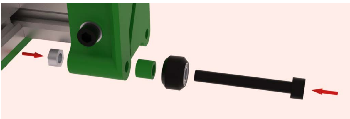
Figure 22: Z Wheel Assembly
